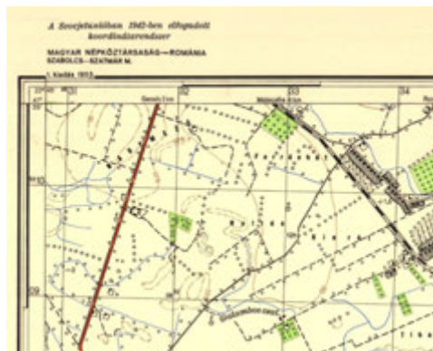
Fig. 26. The map sheet boundaries of the Gauss-Krüger system follow the parallels and meridians.
