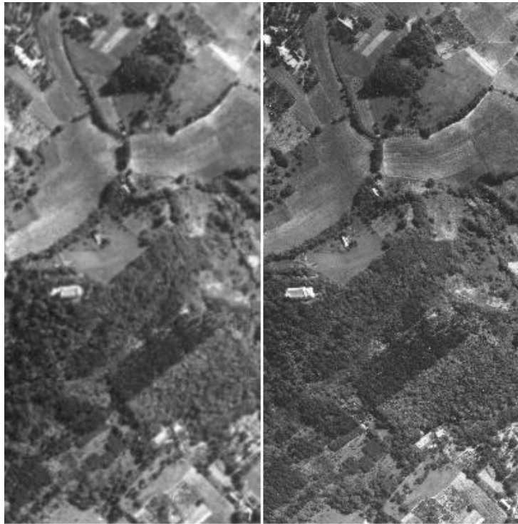
Fig. 48. Stereo photo-pair: if our eyes are focusing to the infinite seeing this, the image appears in 3D.
