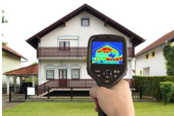
Figure 1.12: Thermography – or infrared scanning – in use to detect thermal defects and air leakage in building envelopes. http://energy.gov/energysaver/articles/thermographic-inspections
